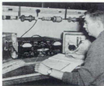
VITRAMON,® Inc., uses the Impedance Comparator for comprehensive measurements on statistical samples from each production lot of capacitors.
